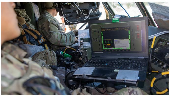
U.S. Soldiers assigned to 2nd Battalion, 20th Field Artillery Regiment, work with the Autonomous Multi-Domain Launcher (AML), on a Palletized Load System (PLS) using a Remote Interface Unit (RIU) as a part of Project Convergence 22 at Fort Irwin, California, Oct. 31, 2022. (U.S. Army /Collin S. MacKown)
