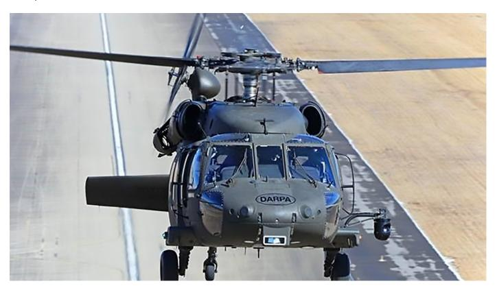
DARPA's Aircrew Labor In-Cockpit Automation System program completed the first flight without a pilot onboard an UH-60A Black Hawk helicopter. (Image courtesy of DARPA)
